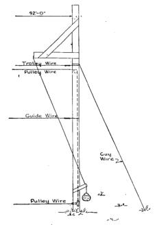
FIGURE 44.—Bumper and wire arrangement.
